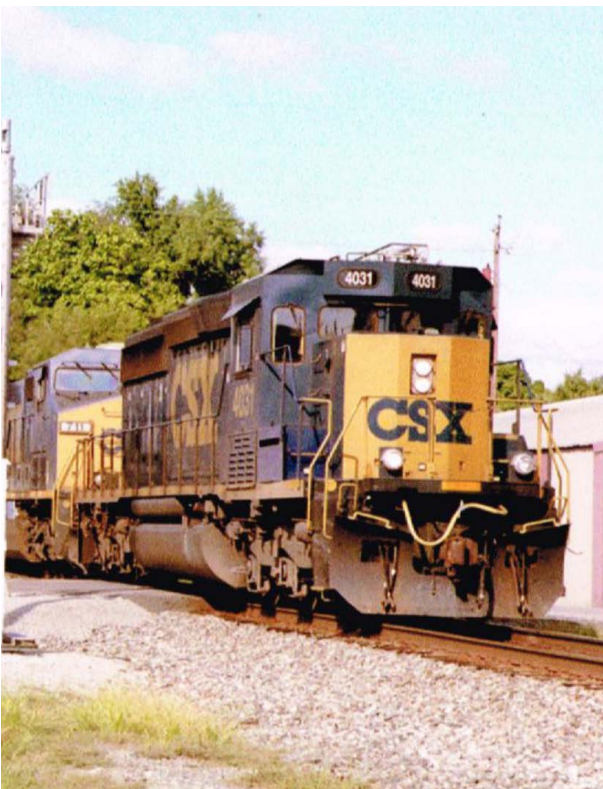
Above: Southbound coal train U-101 led by SD40-3 #4031 rebuilt by CSX from SD40-2 #8143 with new cab and short hood. (There are only 50 of these and they are hard to catch in a lash up and especially on the point.)
